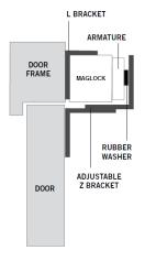
This architectural bracket set for slim maglocks is double covered, giving the smartest appearance possible to the installation of an inward opening door. The fully adjustable Z bracket enables precise alignment of the armature plate with the magnet.
